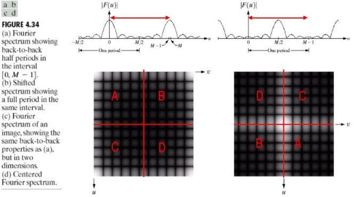
[0, M - 1].(b) Shifted spectrum showing a full period in the same interval. (c) Fourier spectrum of an image, showing the same back-to-back properties as (a), but in two dimensions. (d) Centered Fourier spectrum.
