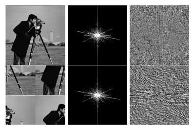
The shift in f(x,y) does not affect the magnitude of its Fourier transform.
