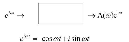
Thus we can understand what the system (e.g filter) does to the different components (frequencies) of the signal (image)
