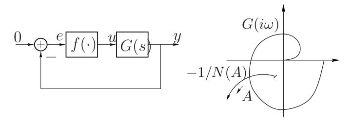
$$y = G(i\omega)u = -G(i\omega)N(A)y \quad \Rightarrow \quad G(i\omega) = -\frac{1}{N(A)}$$
