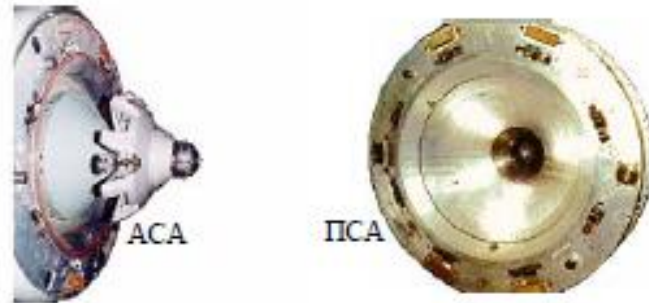
Figure 7.6.2. Active Docking Assembly (ACA) and Passive Docking Assembly (PCA)
