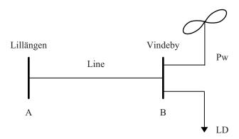
Vindeby is a rather windy area and there is a large potential to install wind power plants. The problem is that the grid is rather weak, which means that there can be large voltage variations for the consumers in Vindeby if too much wind power is installed. The aim of this assignment is to estimate the amount of wind power that can be installed in Vindeby, without violating the voltage requirements.
