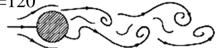
Oscillating Karman vortex street wake (C)
