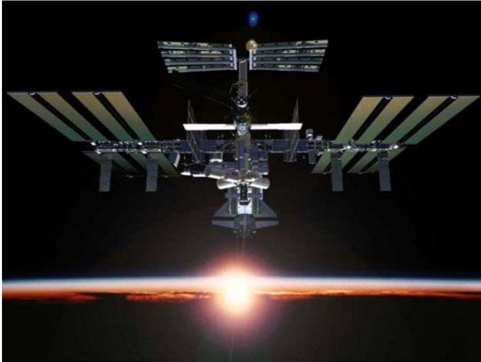
The ISS-station where the solar cells has a power of 250 kW
