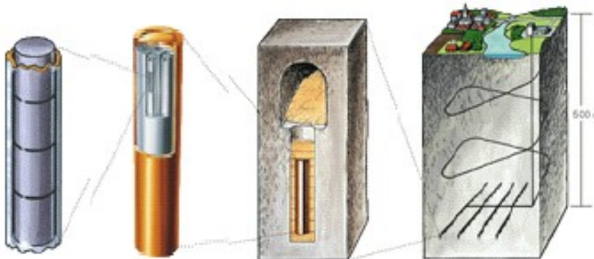
Example of how CLAB will dispose the used nuclear fuel in the bedrock around 600 m below the surface.
