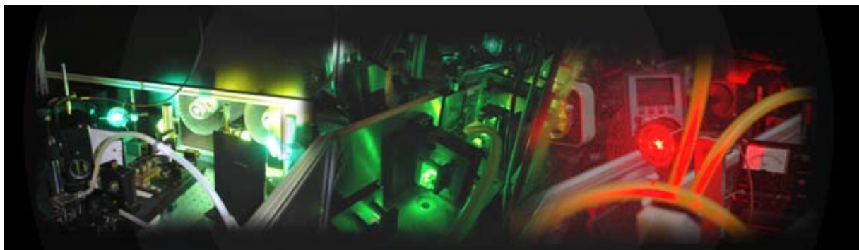
Laser radiation from a copper vapour laser, Nd:YAG-laser and a dye laser
