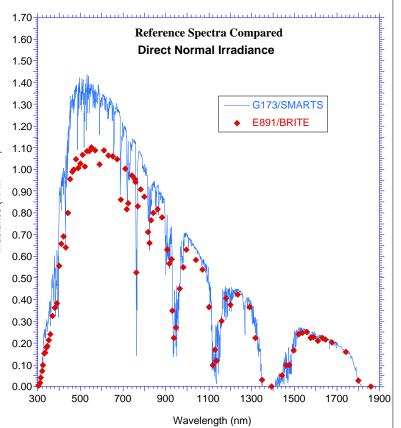
Fig. 2: The new (G173; continuous line) and old (E891; diamonds) reference spectra for direct normal irradiance.
