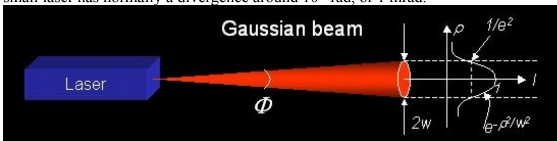
A Gaussian laser beam showing the 1/e 2 point where r = w
