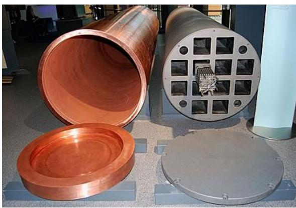
Researchers at KTH have found evidence that the copper canisters may corrode far too rapidly. The estimated service life of 100,000 years for the canisters may as short as less than 1,000 years. The
