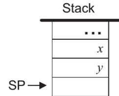
**Figure 7.5** Arithmetic and logical stack commands.
