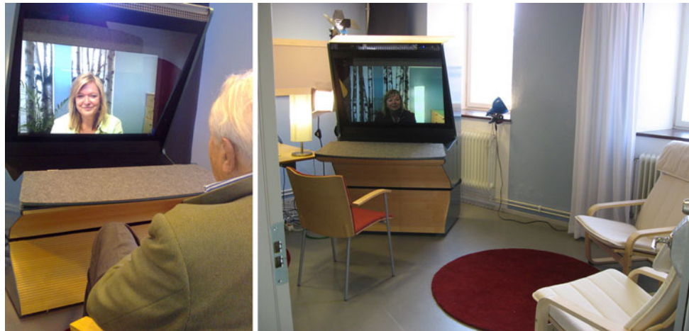
Fig. 10 The mediated consulting room with the piece of furniture designed to enable mutual gaze by incorporating reflective mirrors. To the right, a sitting area where the initial doctor–patient encounter
