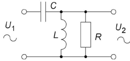
$$a) \quad L \parallel R = \frac{j\omega L \cdot R}{R + j\omega L} \quad \frac{\underline{U}_2}{\underline{U}_1} = \frac{\frac{j\omega LR}{R + j\omega L}}{\frac{1}{j\omega C} + \frac{j\omega LR}{R + j\omega L}} \cdot \frac{(R + j\omega L)j\omega C}{(R + j\omega L)j\omega C} = \frac{\omega^2 RLC}{R(\omega^2 LC - 1) - j\omega L}$$
