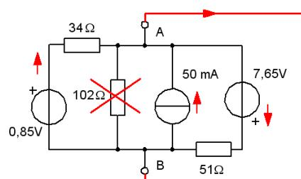
a)  $R_I$  – vrid ner alla  $E$  och  $I$ .  $R_I = 34 \parallel 102 \parallel 51$ .  $R_I = \frac{1}{\frac{1}{34} + \frac{1}{102} + \frac{1}{51}} = 17 \Omega$
