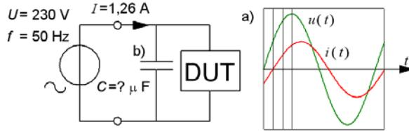
a)  $\varphi = 30^\circ \quad \cos(\varphi) = 0,866 \quad P = UI \cos \varphi = 230 \cdot 1,26 \cdot 0,866 = 250 \text{ W}$
