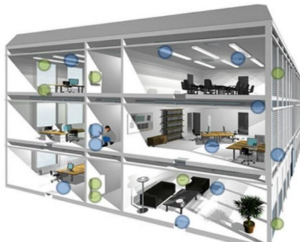
WSNs for controlling temperature, light, air and humidity, doors, alarms
