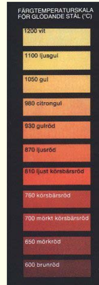
Chart to estimate steel temperature in steelworks.
