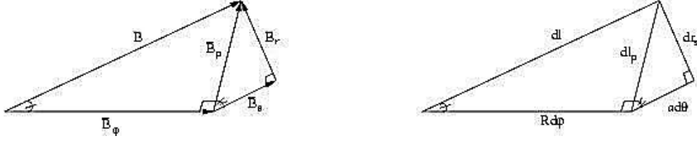
Figure 2: The triangles show the relation between the magnetic field vectors and the flux surface displacement.
