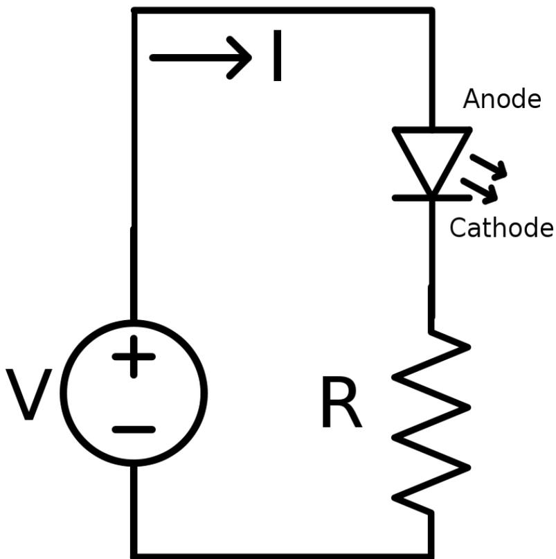
As a more complex example we would like to light a LED (light-emitting diode) from an output pin on an embedded computer. Consider that our output pin can source 20mA at +5V. Our LED is green, which implies a forward voltage drop of about 2 V. However, we also need to consider that our LED requires at least 10mA to light, and our LED can not exceed +20 mA. If the current through the LED gets too high, the LED could pop (it's an actual pop, cover your eyes).
